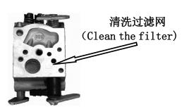
NOTICE: The carburetor fuel screen should be cleaned periodically also. Carefully remove the pump cover (inlet side of the carburetor), gasket and pump membrane. The screen will be visible and can be cleaned after careful removal.
