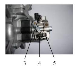
(1)、风门,冷启动时使用; Choke Arm (The Choke Arm is used under the circumstance of cold start-up.); (2)、油门; Throttle; (3)、 怠速调节螺丝; Idle Adjustment Screw; (4)、低速油针; Low-speed Needle; (5)、高速油针; High-speed Needle;
