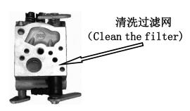
NOTICE: The carburetor fuel screen should be cleaned periodically also. Carefully remove the pump cover (inlet side of the carburetor), gasket and pump membrane. The screen will be visible and can be cleaned after careful removal.
